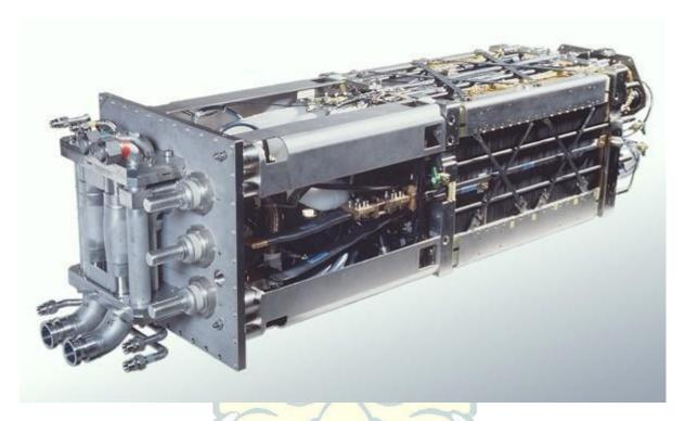
Phosphoric Acid Fuel Cells (PAFC) and Proton Exchange Membrane Fuel Cells (PEMFC) are presently used in submarines. Germany is said to be the world leader in developing and fielding this type of AIP, which is backed by the large number of export orders they have received. France is developing a new generation Fuel Cell AIP as a successor to its MESMA. India is another country which is developing a Fuel Cell AIP to be integrated on their submarines.
